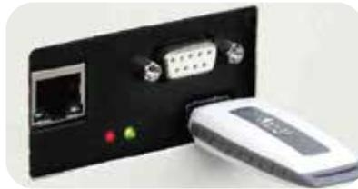
**USB flash disk storage.** Timely sterilizing information storage to guarantee all data can be safely stored and traced during the sterilizer service life. This configuration can also be updated to a traceability system.
